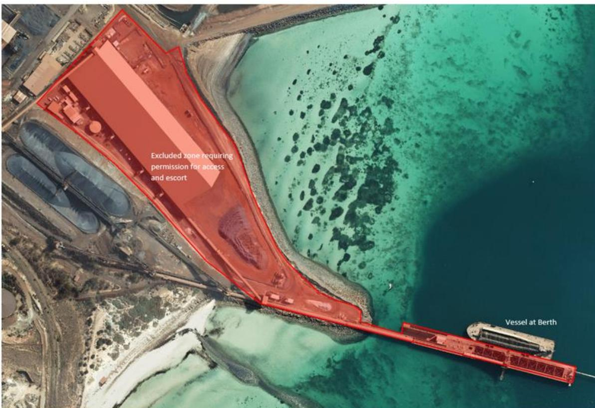
The Outer Harbour consists of a channel, an Ore Jetty known as the Outer Harbour Transshipment Berth (OHTB) and a Swing Basin.
