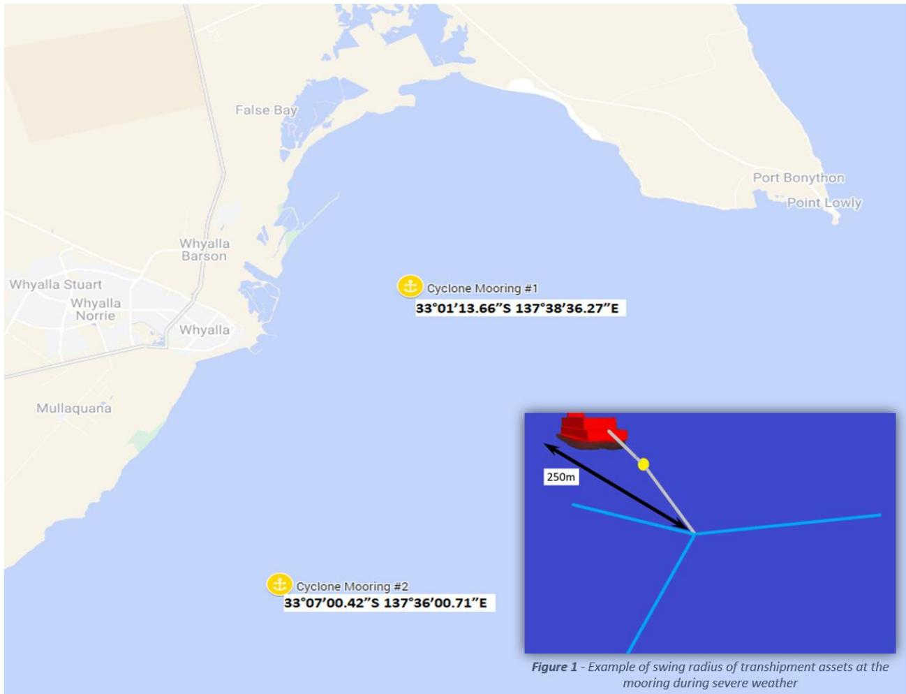
Figure 1 - Example of swing radius of transhipment assets at the mooring during severe weather
