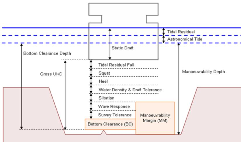
Figure 3 Maximum sailing draft - static calculation method
